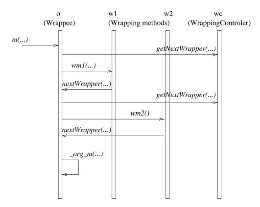
Figure 4: The wrapping control mechanism.
